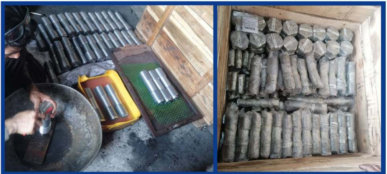
Turbine Fasteners GE HYDRO (Mangla Power Station)
