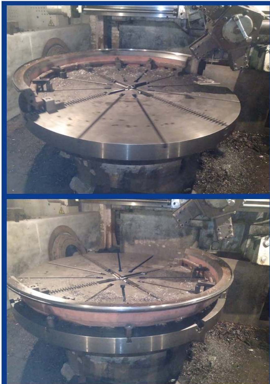
Machining of Support Ring OD: 96 inch GE VERNOVA (Bhikki Power Plant)
