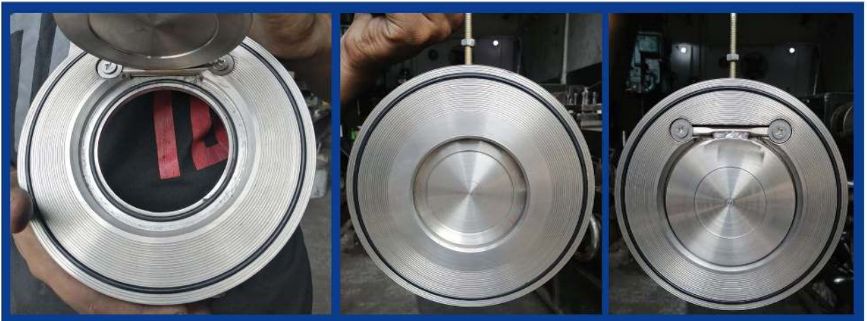
NRV for Cooling Tower Line HUBCO (Narowal Energy Limited)
