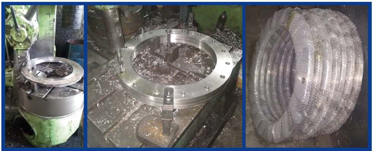
SS Gaskets for Expansion Joints GE VERNOVA (THAL-NOVA Project Tharparkar)
