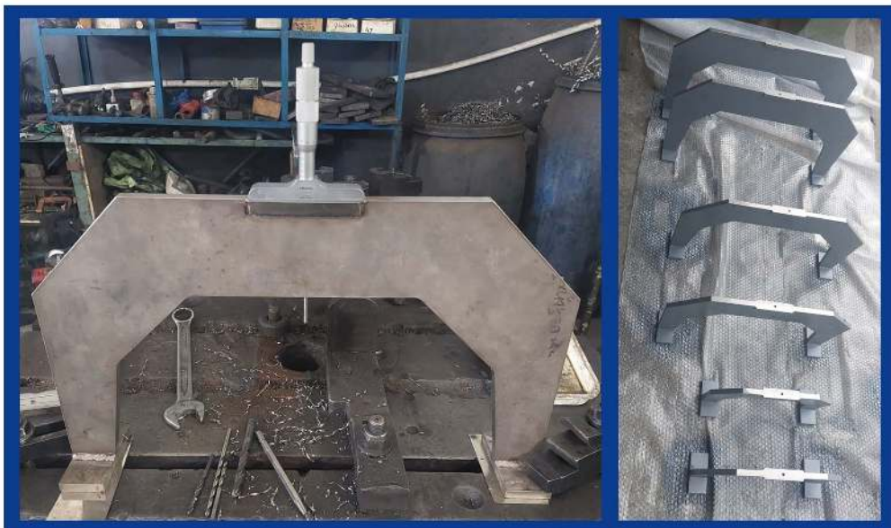
Fabrication of Bridge Gauge to measure Turbine Journal Bearing Clearance GENERAL ELECTRIC (Lucky Electric Company)
